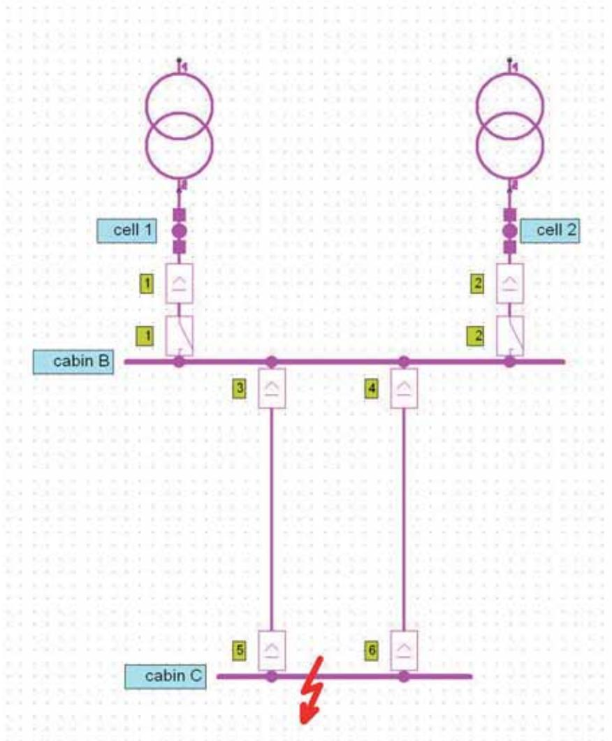
Figure 5 : Fault location in the grid
