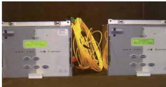
Figure 3 : Protection relays
